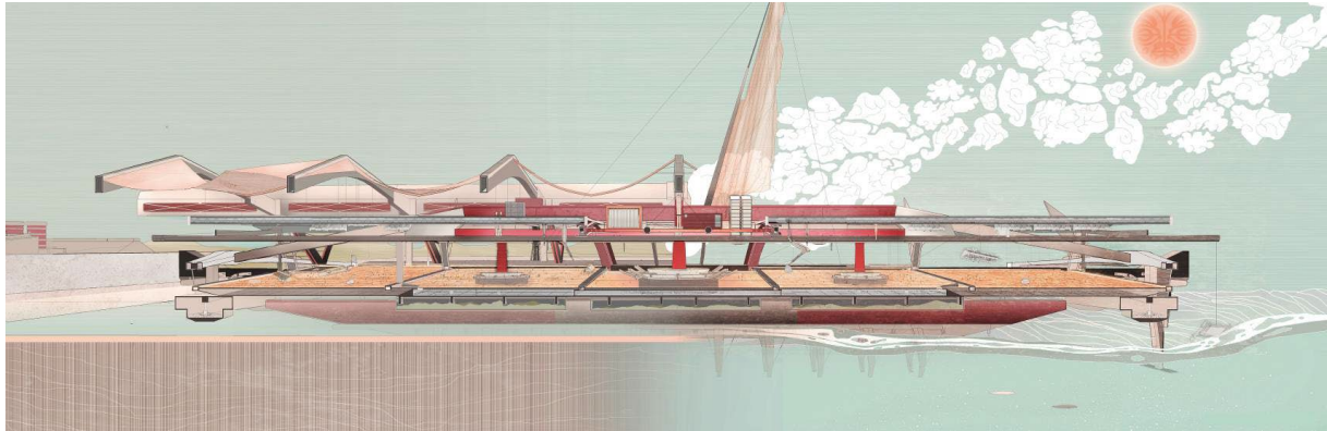
Fig.15: Sectional drawing of Lomipeau showing two modes of operation: Land mode (left) where the canoe is attached to the Afolau, and the Voyage mode (right) which gains Lomipeau mobility
