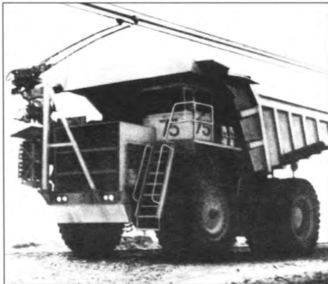
Fig. 4: Trolley truck operating at the Quebec Cartier iron ore mine, Lac Jeannine, 1970s.
